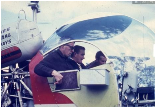
Large double-ended matches or Delayed Action Incendiary Devices (DAIDs) were struck on the striker pad on the side of this Bell 47G helicopter and dropped by hand. DAIDs were kept in a box on the outside of the door with a quick-release mechanism. The rate of ignition approximately 300 acres per hour. Photo: Grange Jephcott.
