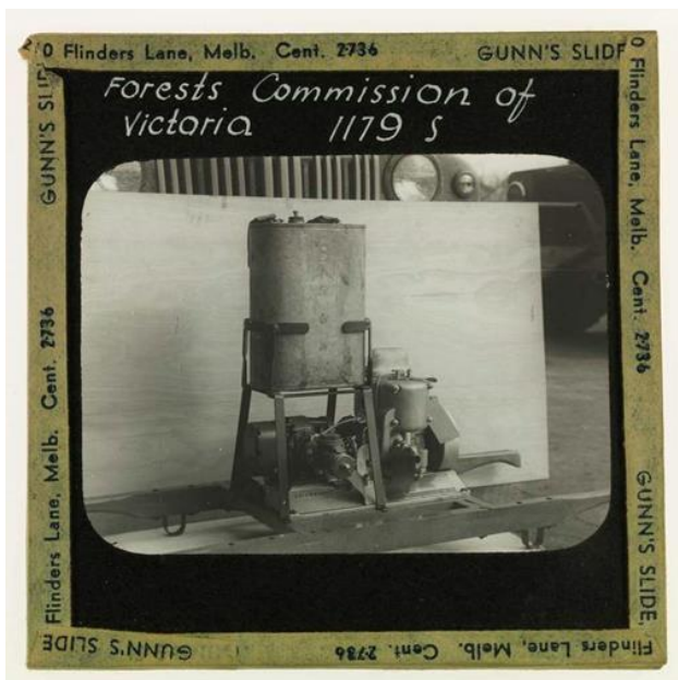
The cantankerous high-pressure Type Y Pacific marine pump. A bummer of a thing to start and always guaranteed to take the skin off your knuckles. They had a very high fuel-oil mix so blew great clouds of smoke and screamed at high revs.
