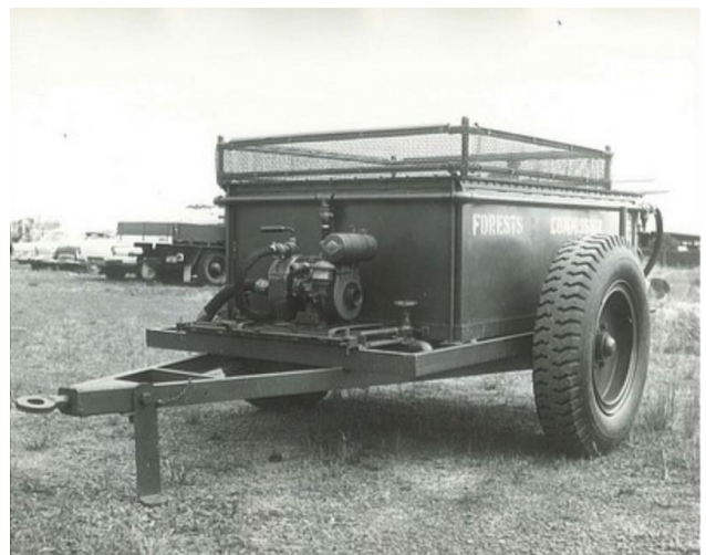
Trailer water tanks that were fitted with a pump and hose racks were developed at Altona in the 1960s. Source: Barry Marsden.
