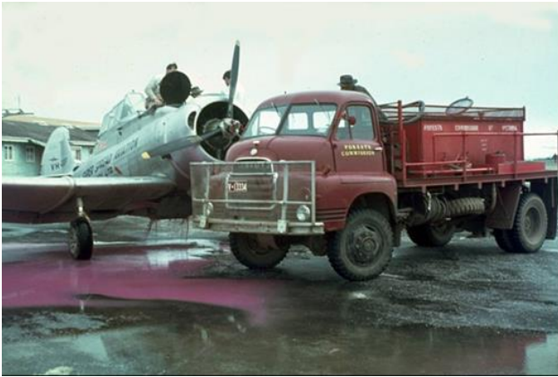
Firebombing trials at Ballarat dropping water thickened with bentonite clay from a CRC Ceres CA-28 aircraft – 1962. Photo: Athol Hodgson.
