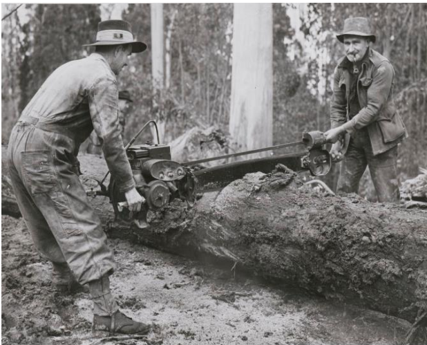
The advent of petrol-powered chainsaws after WW2 revolutionised both logging and firefighting. This two-man saw is an American manufactured Mercury Disston. The 11Hp model with a 36-inch bar weighed a massive 102 pounds or 46kg whereas a comparable Stihl 880 weighs about 14kg. Source: State Library of Victoria - circa 1948.
